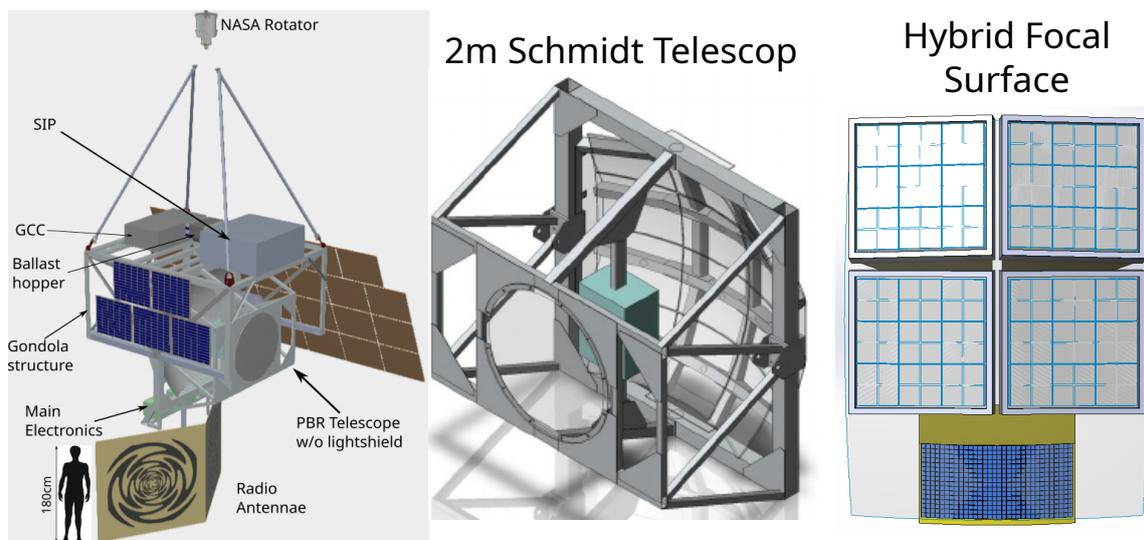
**Figure 2:** Left: Design of the PBR payload. Center: Mechanical drawing of the telescope structure. Right: Drawing of the Hybrid focal surface consisting of the FC and the CC.
