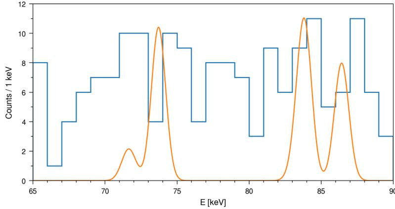
**Figure 2:** Spectrum acquired with the germanium detector in the VIP-Lead experiment, in about 70 days of data taking. The expected signal distribution is shown in orange with arbitrary normalization. Reproduced from [12].
