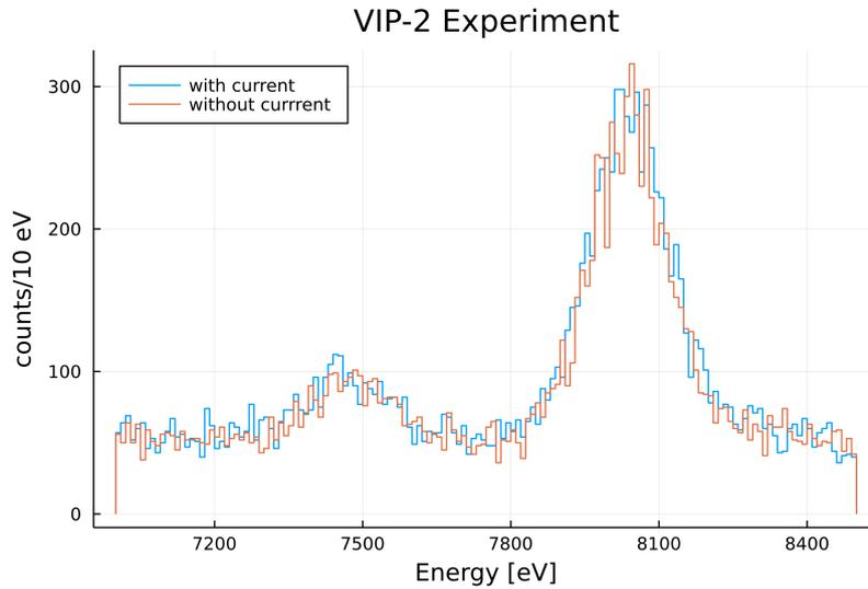
**Figure 1:** Spectra acquired with current on (blue) and off (orange) by the VIP-2 experiment in approximately six months of data taking in the Region of Interest 7000-8500 eV. The two peak are the nickel  $K\alpha$  and the copper  $K\alpha$  lines, while the signal is expected at around 7700 eV. Reproduced from [9].
