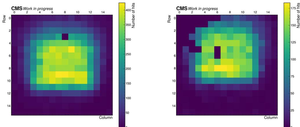
**Figure 3:** Number of hits collected per pixel for labeled ETL test modules 36 and 37 obtained during a run of the SPS test beam in May 2024.
