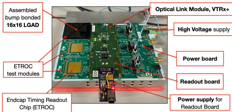
**Figure 1:** Photo of the ETL module testing setup showing three ETL custom test boards connected to a readout board. The readout board is connected to an optical link module VTRx+ coupled to a fiber. The upper test boards has an assembled 16x16 LGAD bump bonded to an ETROC. Low voltage is supplied to the modules either through the readout board or by an external power board, while high bias voltage is provided externally.
