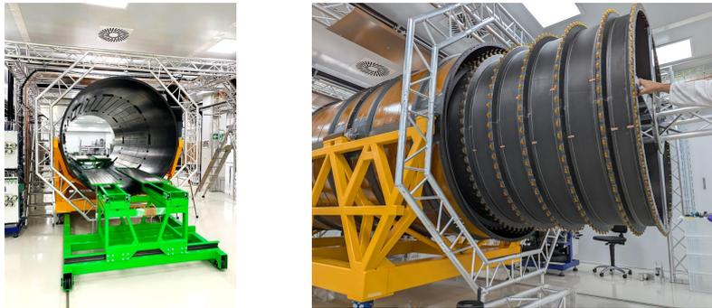
**Figure 3:** Assembly of the outer cylinder started in June 2024 (left). The Strip Layer 3 cylinder also arrived at CERN for insertion inside the outer cylinder. The first insertion tests have been performed successfully in July 2024 (right).
