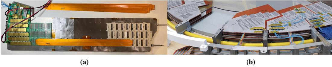
**Figure 5:** (a) Assembled demonstrator used for system-level integration tests. (b) Mock-up setup for validating installation methods.
