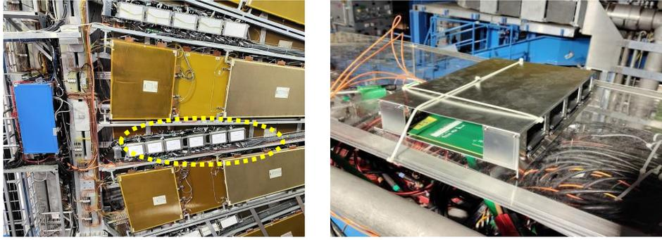
**Figure 6:** Photographs showing the demonstration of actual installation of phase-2 frontend electronics for TGC, including board placement and cablings (left), and electronics demonstrators installed in the ATLAS cavern (right) to validate communication links and measure the single event upset rate on the FPGA during Run-3 operations.
