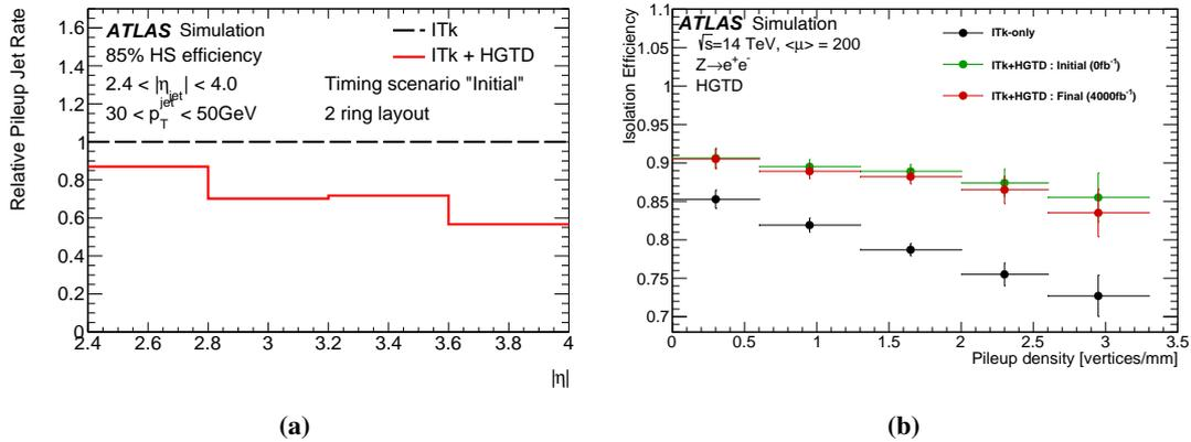
**Figure 4:** (a) Relative rate of pileup jets as a function of jet pseudorapidity ( $\eta$ ) for jets with  $30 < p_T < 50$  GeV. (b) Efficiency for electrons to meet track isolation criteria as a function of local vertex density, comparing the ITk-only and ITk+HGTD configurations. The plot shows performance for two timing resolution scenarios, representing the beginning and end of HL-LHC operation [5].
