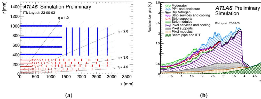
**Figure 1:** (a) A schematic illustration of the ITk system, where the components of the strip detector are depicted in blue, and those of the pixel detector are depicted in red. (b) The material distribution within the ITk volume is shown in radiation lengths ( $X_0$ ) as a function of pseudorapidity ( $\eta$ ) [4].
