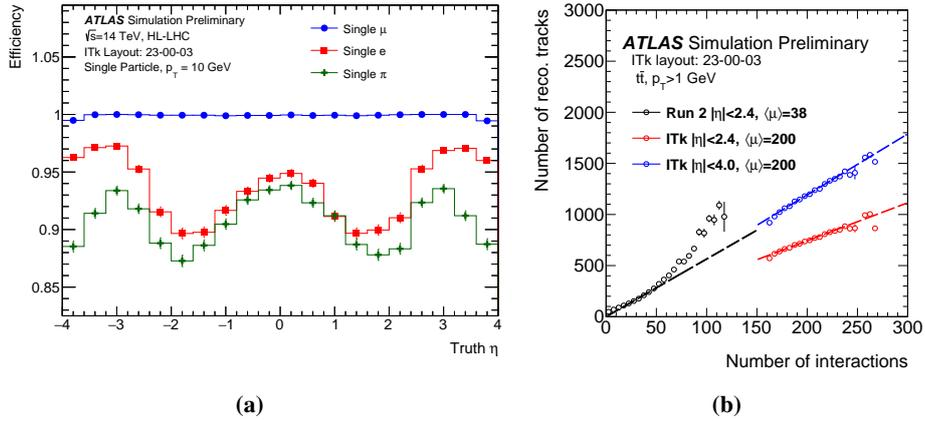
**Figure 2:** (a) Tracking efficiency for individual particles with  $p_T = 10$  GeV is shown for muons, electrons, and pions, without pileup effects. (b) The number of reconstructed tracks per event with  $p_T > 1$  GeV is displayed for  $t\bar{t}$  events, with an average of 200 pileup collisions, as a function of the actual number of interactions. For comparison, results are shown for the Run-2 detector geometry using the Run-2 legacy reconstruction software [4].
