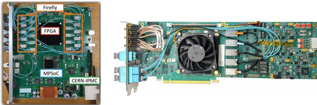
**Figure 7:** Photographs of prototypes for the Level-0 Muon Trigger Sector Logic electronics in ATCA form factor (left) and the FELIX PCIe card for the readout in the Phase-II system with extended input bandwidth (right) [9].
