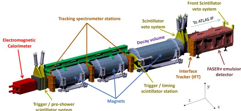
**Figure 2:** Illustration of the FASER detector design. Reproduced from [8].
