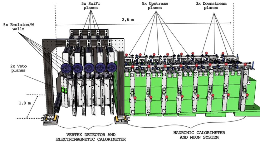
**Figure 1:** Illustration of the SND@LHC detector design. Reproduced from [3].
