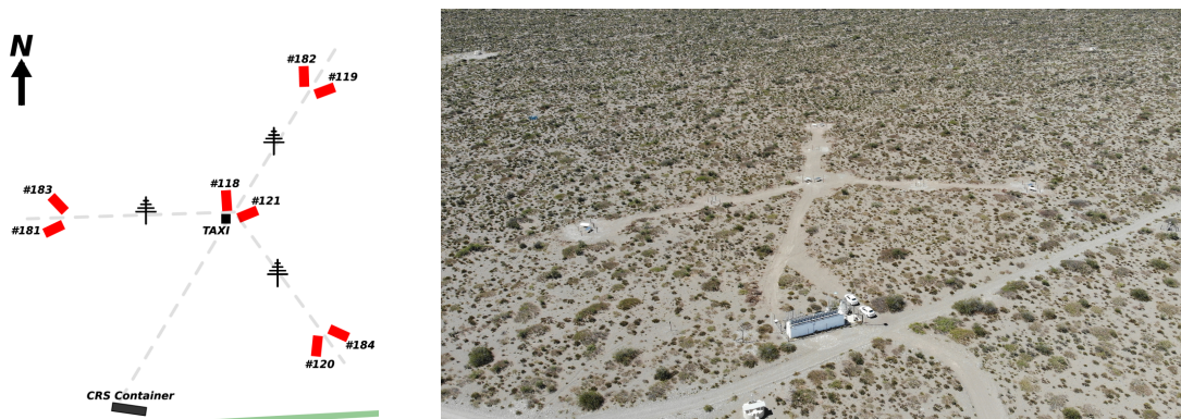
Figure 1: Left: Layout of the prototype detector station. The red rectangles represent scintillator panels, the antennas are shown in black. The central DAQ is represented by the black square labeled “TAXI”. The Central Radio Station of AERA is used for data collection and power supply. Right: Drone shot of the station at the site of the Pierre Auger Observatory (photo by Tim Huege).
