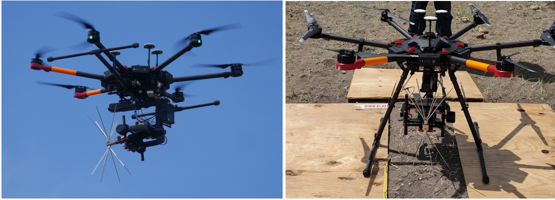
Figure 3: The DJI Matrice M600 Pro together with the calibration equipment mid-flight (left) and stationary (right).
