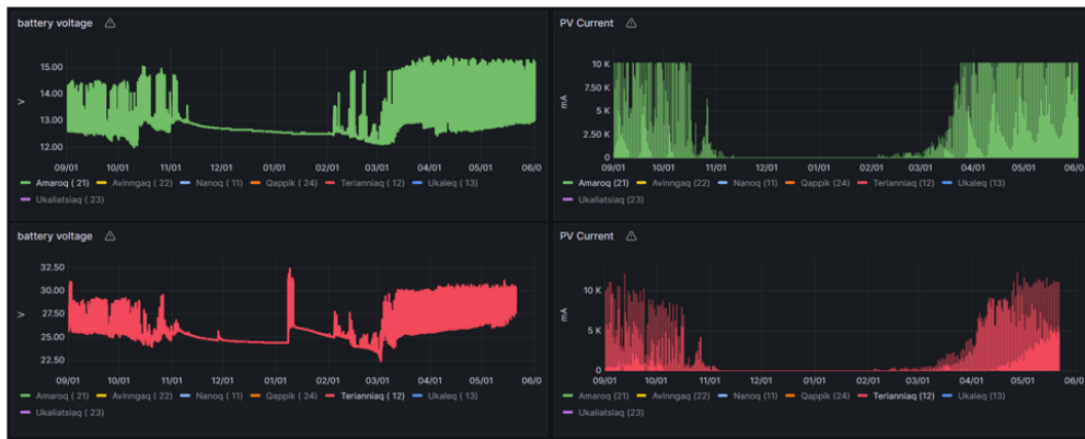
Figure 2: Readout from monitoring tools for a yearly power draw comparison of station 21 with (top, green) and station 12 without (bottom, red) wind turbines. With zero PV current during the winter months, the battery voltage of station 12 shows charging during the winter where no sun is present.
