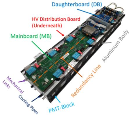
**Figure 4:** Fully equipped mini-drawer
