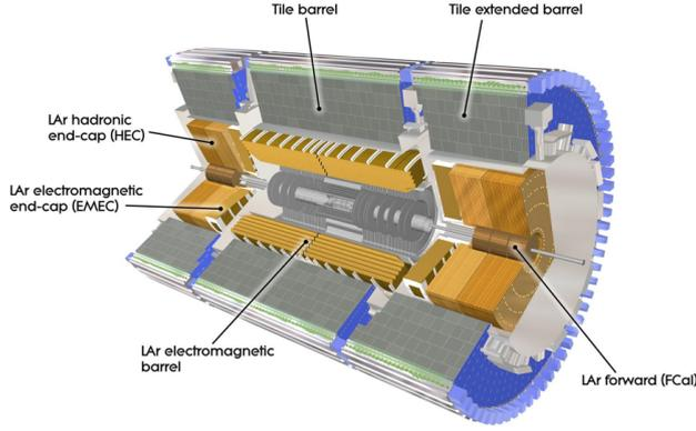
**Figure 1:** ATLAS calorimetry [1]
