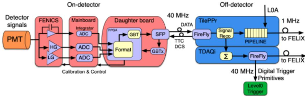
**Figure 3:** Schematic view of the new TileCal electronics architecture
