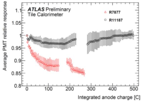
**Figure 5:** Response evolution comparison of PMT models [4].
