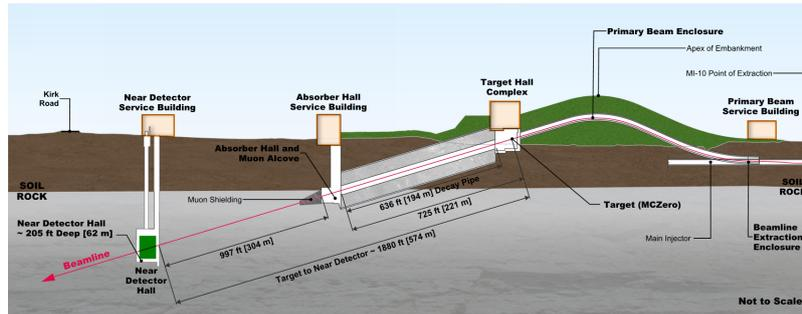
Figure 1: LBNF Beamline from Fermilab, Illinois to South Dakota [6]
