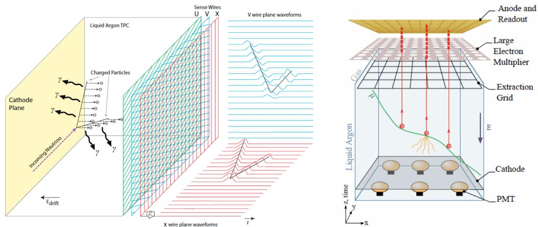
**Figure 7:** Operating principle of Single-Phase technology (Left) and Dual-Phase technology (Right) [6]
