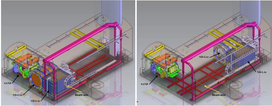
**Figure 6:** DUNE ND with ND-LAr and ND-GAr in the on-axis (Left) and off-axis (Right) beam positions. The SAND detector is shown in beam on-axis position.
