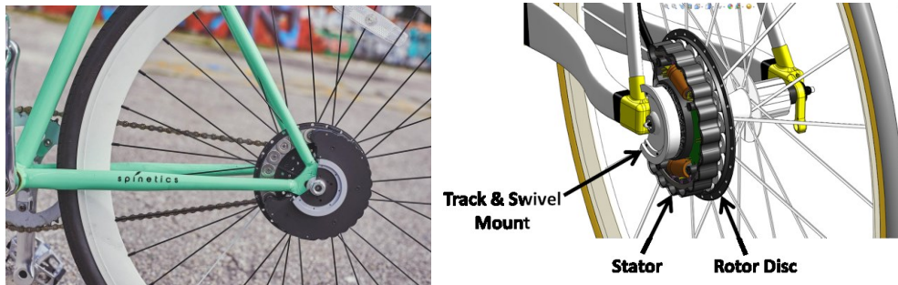
Figure 6: Principle of Micro-Electricity Generation On the left, the Spinetics's Cydekick device, and on the right, the principle of how the device is composed.
