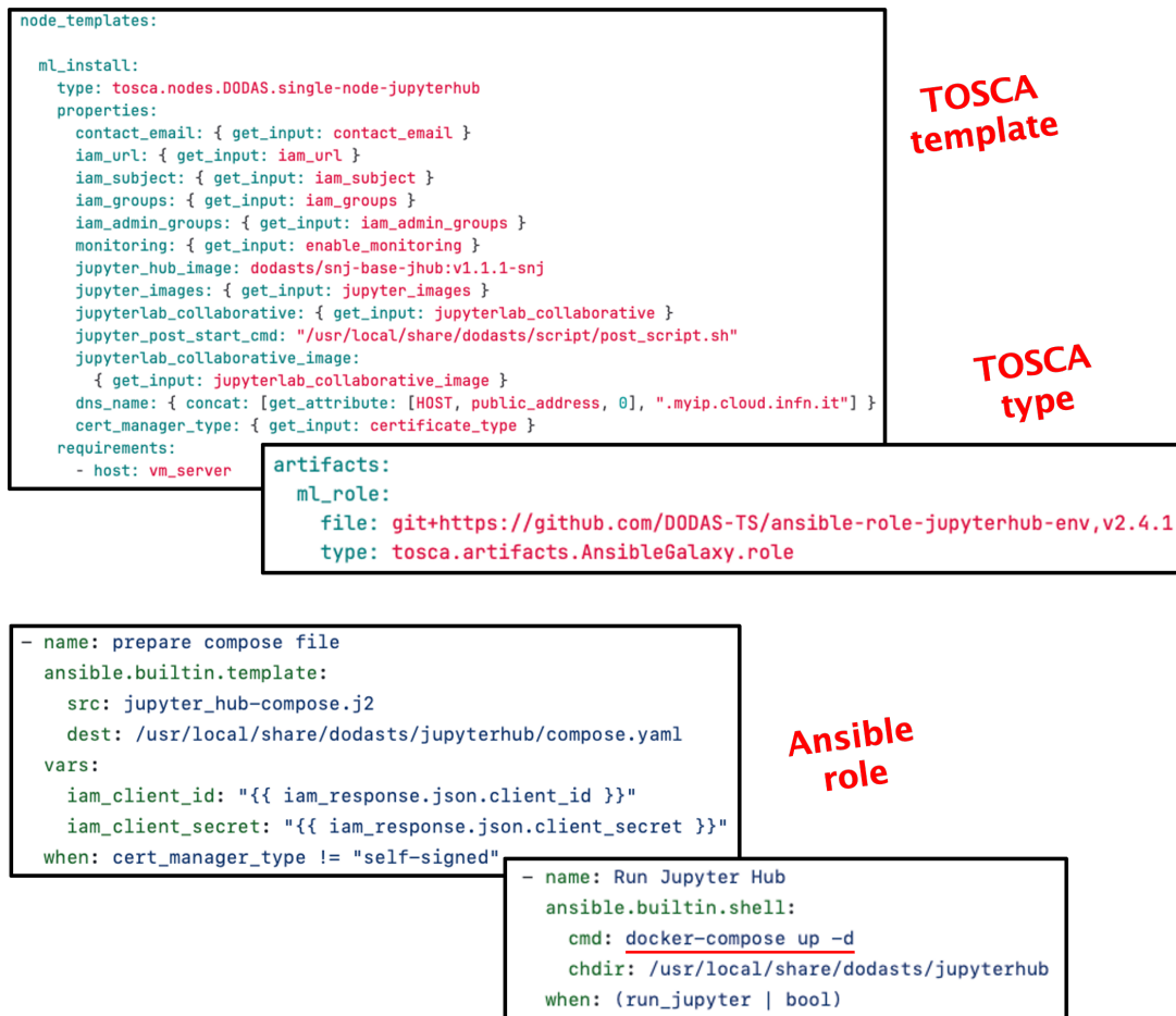
Figure 2: Combination of TOSCA template and type, Ansible role, and Docker containers (run using a Docker compose file created from a Jinja template [10] called jupyter_hub-compose.j2 ) used for the creation of Jupyter with persistence for Notebooks service.
