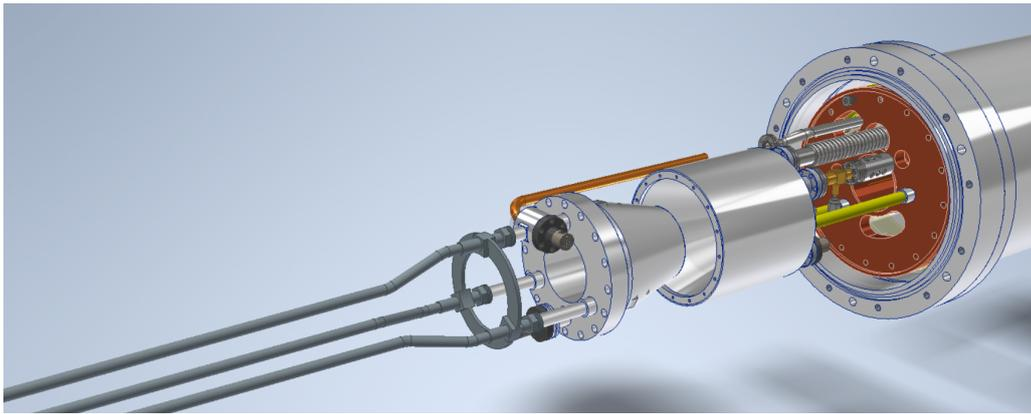
**Figure 5:** Modular, conical heat-exchanger of the Hall B cryotarget. The coolant loop on the right cools the concave conical mount to below 4 K with Joule-Thomson cooling of liquid helium. Extending to the left is the target loop which will support and cool our gas cells. The experimental beam passes through the center bore of the refrigerator.
