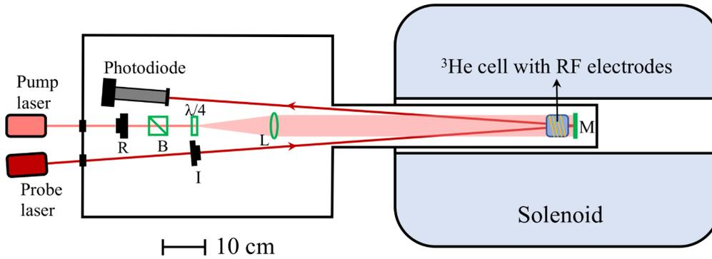
**Figure 7:** Schematic layout of our MEOP test apparatus, from [15].
