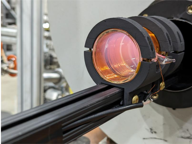
**Figure 1:** Photograph of a sealed helium cell under plasma discharge.
