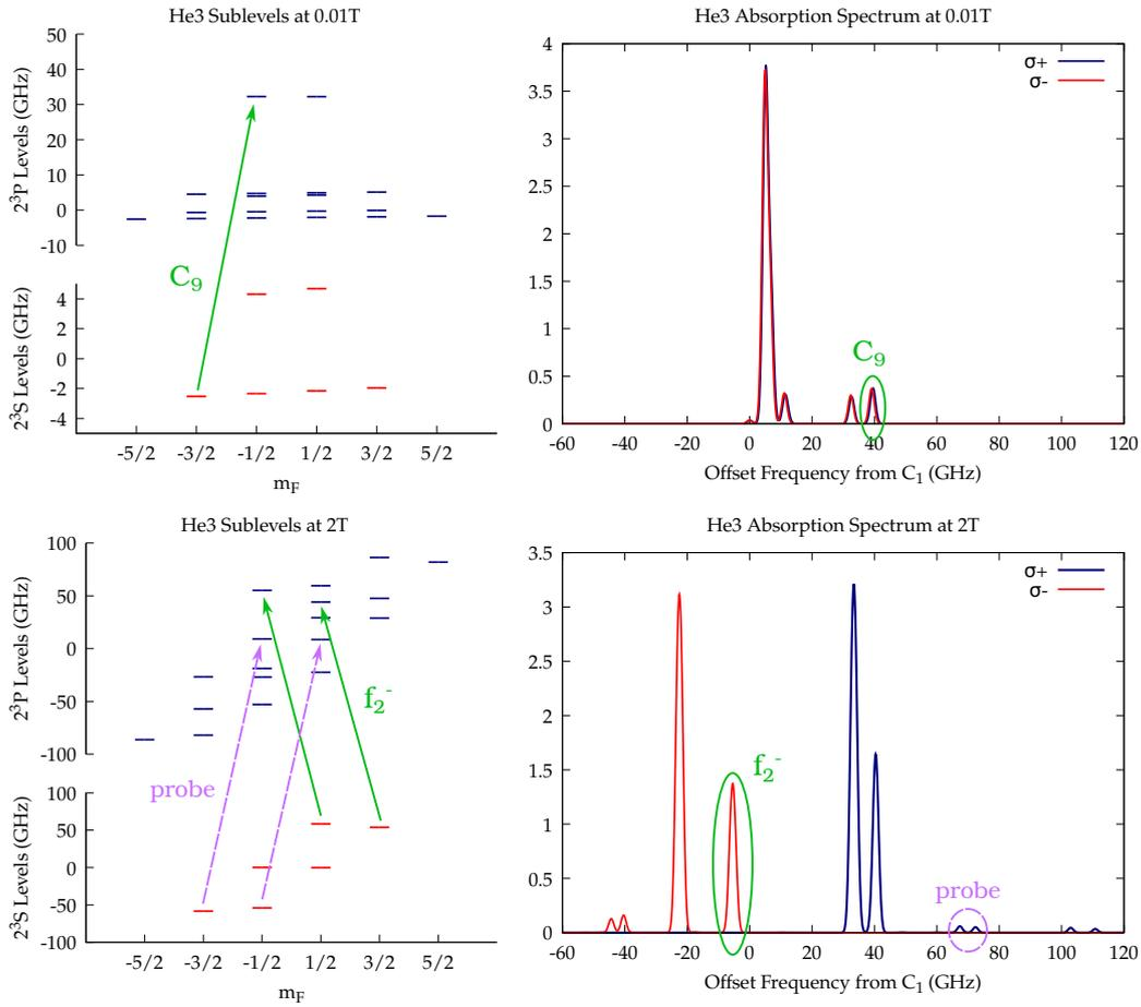
**Figure 3:** Optical pumping transitions at low (top) and high (bottom) magnetic fields. At left are the separations of the  $^3\text{He}$  sublevels, with example pumping transitions  $C_9$  and  $f_2^-$ . At right are the corresponding peaks in the absorption spectrum. Based on figures from [6, 7], calculated using code from P.J. Nacher.
