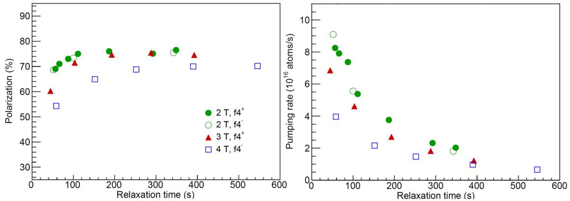
**Figure 8:** At left, the steady-state polarization achieved at JLab from 2 to 4 T with a 1.3 mbar sealed gas cell versus the discharge-on relaxation time with the laser off, and at right the corresponding pump up time with the laser on.
