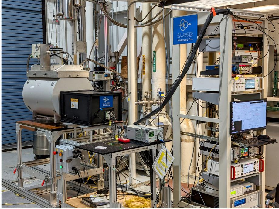
**Figure 6:** Photograph of the laser enclosure (in black) extending into the warm-bore magnet at left, and the supporting electronics rack on the right.
