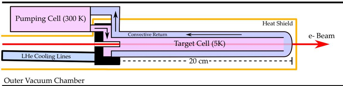
**Figure 4:** Schematic layout of the two-cell polarized  $^3\text{He}$  target concept for CLAS12, from [11].
