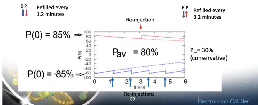
Figure 2: EIC beam polarization and intensity vs. time [18].
