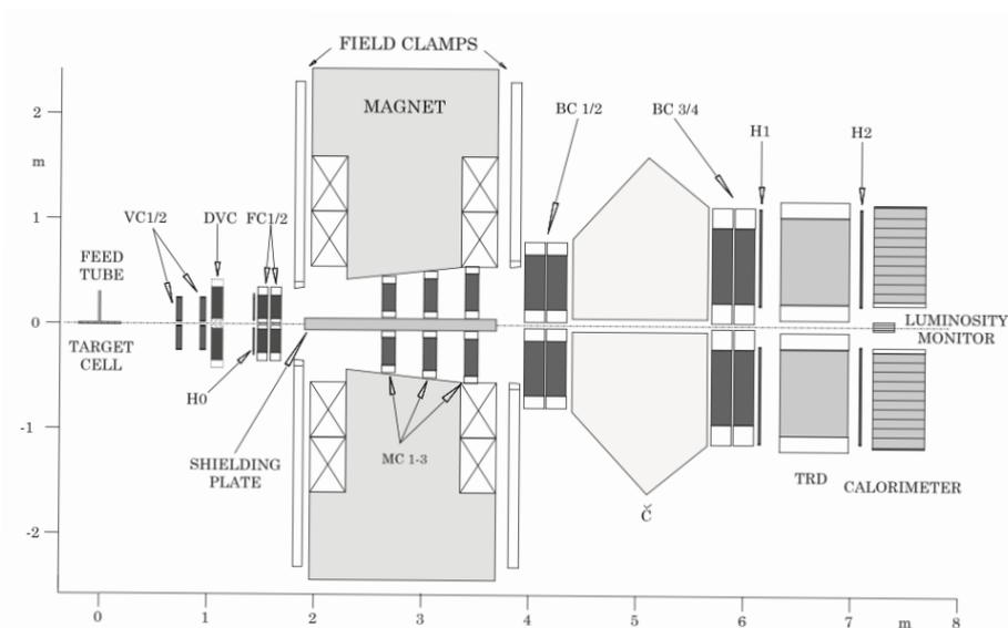
Figure 3: Layout of the HERMES spectrometer [20].
