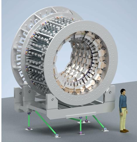
**Figure 3:** CAD layout of the MOLLER main integrating detector [11].
