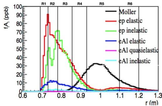
**Figure 4:** The average asymmetry distribution of simulated signal and backgrounds at the main detector. The Møller electron signal is in black, elastic scattering on the proton is red, inelastic scattering from the proton in green, and elastic, quasielastic, and inelastic scattering from the Al target windows in blue, magenta, and cyan, respectively. The figure is taken from [3].
