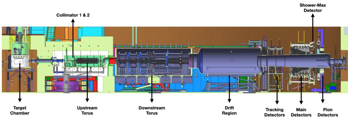
**Figure 2:** CAD layout of the MOLLER experimental apparatus [4].
