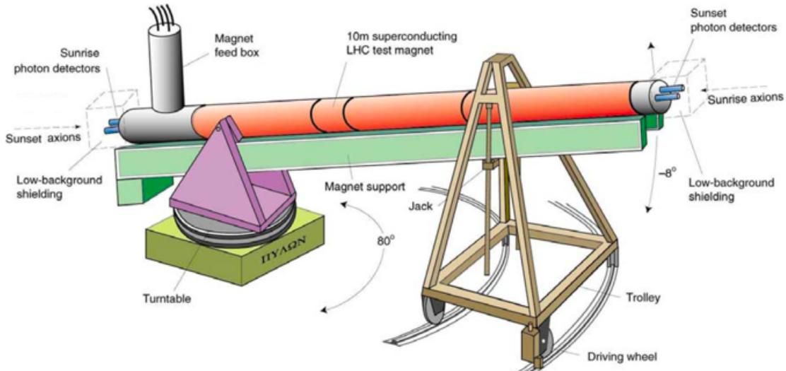
**Figure 1:** Drawing of the CAST magnet and the movement system.
