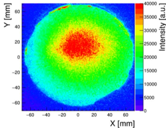
**Figure 2:** A beam profile of surface muons measured with a beam profile monitor at the H1 area
