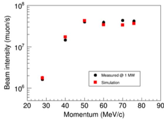
**Figure 3:** Negative muon yields measured with several momentum settings. The black circles are measured intensities and the red squares are the results of simulation.
