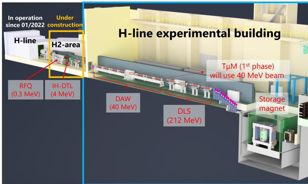
Figure 4: A 3D drawing of the extension plan of the H-line.
