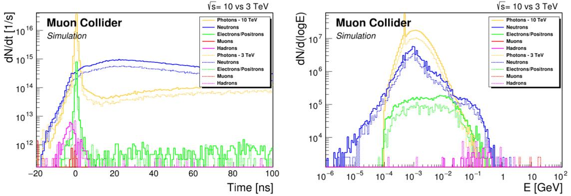
**Figure 3:** Left: Distribution of the arrival time of particles arriving at the detector for  $\sqrt{s} = 3$  TeV (dashed line) and  $\sqrt{s} = 10$  TeV (solid line). Different colors represent different particle types. Right: Energy distribution of the same particles in the same conditions but in the time window [-1 15] ns.
