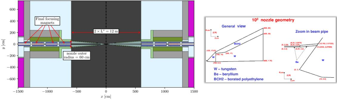
**Figure 2:** Left: IR of the 10 TeV center-of-mass energy, the  $x$  axis represents the beam direction. The outer shape of the detector is a cylinder with a radius of 6 m. The space between the outer shape and the nozzles is considered as a perfect particle absorber. Right: MAP nozzle design [6].
