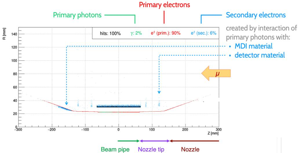
**Figure 4:** Origin of beam-induced background hits in the first layer of the tracker. Particles coming from the IR including nozzles are labeled as primary while those originating in other material are called secondary. One muon beam coming from the direction of the peach-coloured arrow is used. The different location of the machine-detector interface elements is described on the bottom of the figure. A symmetrical configuration can be assumed for the other muon beam.
