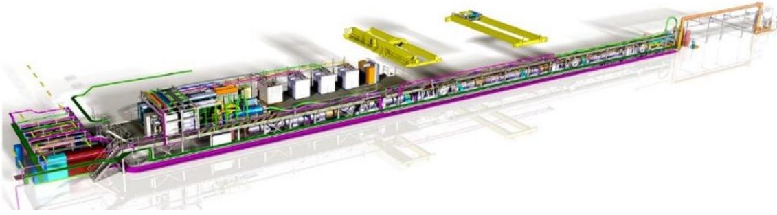
**Figure 6:** Inner Triplet String under installation in CERNs SM18 test facility. Magnet string from Q1 to D1 is located on the ground floor, while all powering and protection equipment is housed on a metallic platform.
