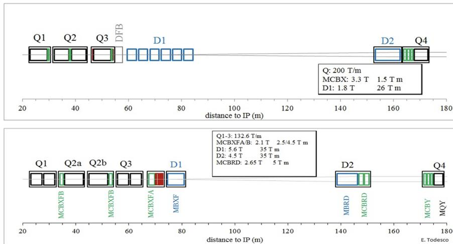
Figure 2: Layout of the insertion region magnets in present LHC (top) and HL-LHC (bottom)
