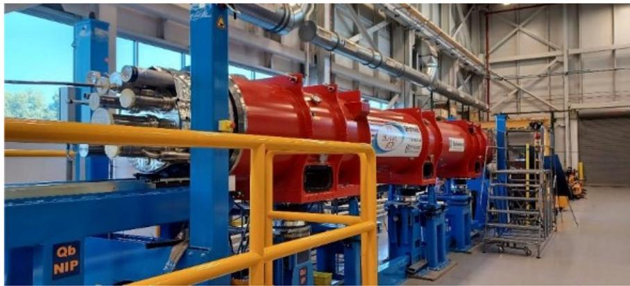
Figure 3: First inner triplet quadrupole cryoassembly of the AUP collaboration
