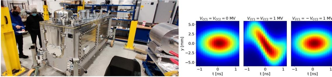
**Figure 5:** Cryostated assembly of 2 RFD CCs, being prepared for shipment to CERN and later installation in the SPS (left). Crabbing of proton bunches in the SPS in 2018 (right).
