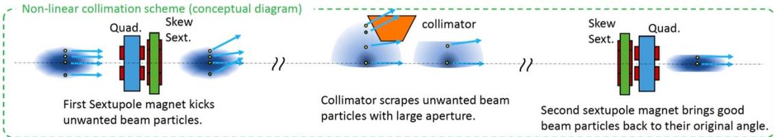
Figure 10: Non-linear Collimation scheme with a set of skew sextupole magnets.
