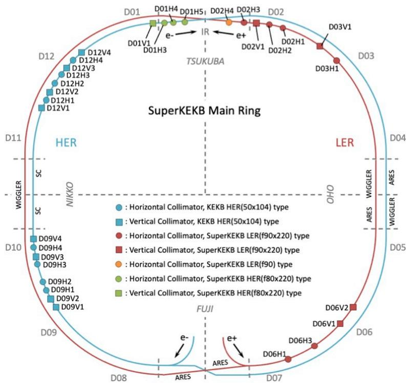
Figure 3: SuperKEKB collimator locations for HER and LER. V and H indicate vertical and horizontal collimators, respectively.
