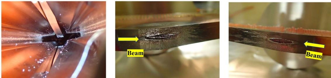
Figure 5: Damaged collimator heads by a direct hit by beam.
