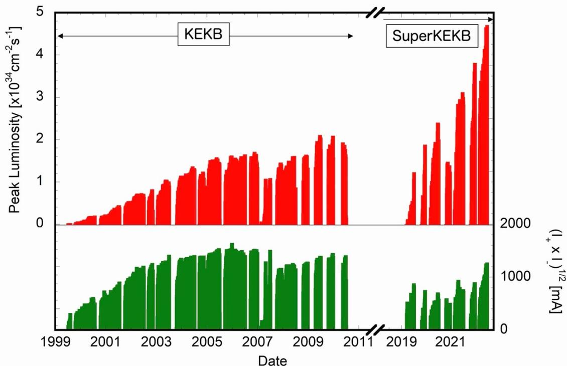
Figure 1: Peak luminosity achieved (top) and the average of the beam currents in the HER and LER for KEKB and SuperKEKB, respectively.
