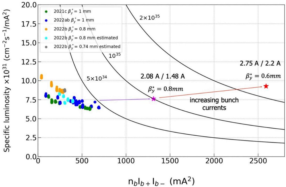
Figure 11: Luminosity plotted against the product of beam currents for different  $\beta_y^*$ .
