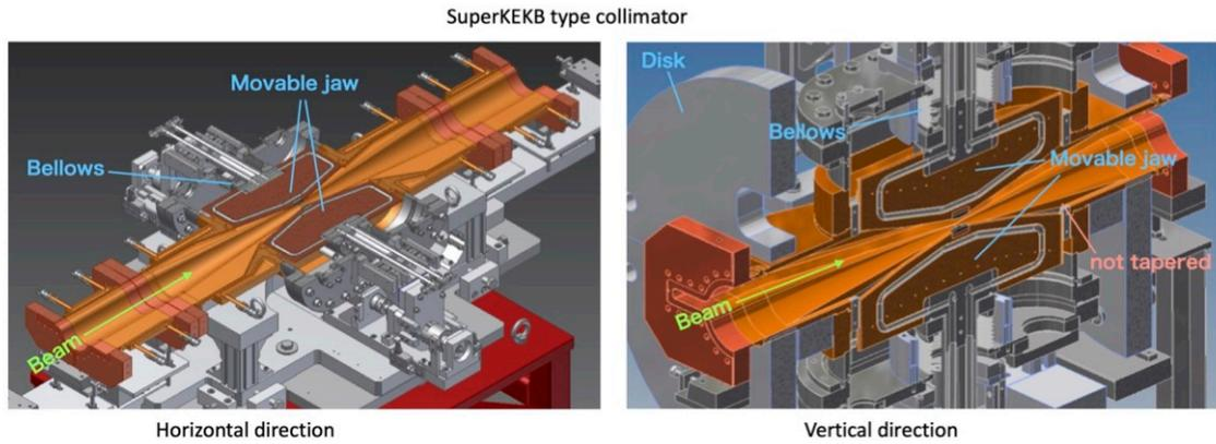
Figure 4: SuperKEKB horizontal (left) and vertical (right) collimators, movable jaws are controlled remotely.
