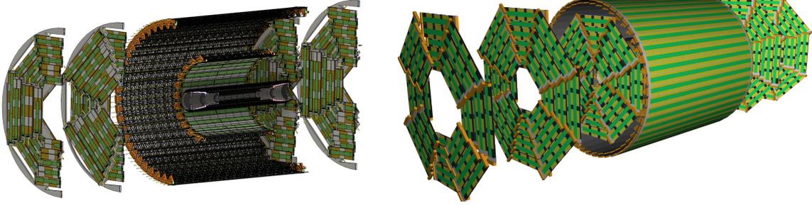
**Figure 2:** CAD model (left [3]) and DD4hep implementation (right) of the IDEA vertex detector.
