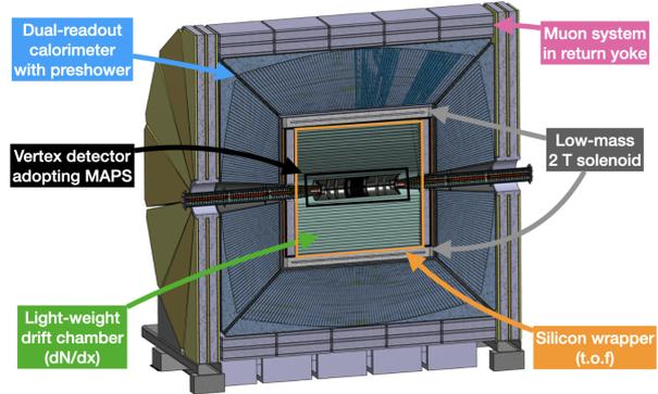
**Figure 1:** The IDEA detector concept for FCC-ee.
