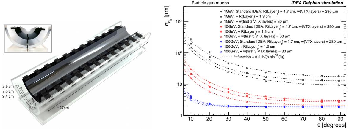
**Figure 4:** Mechanical prototype of the ALICE ITS3 detector [4] (left) and effect of reduced material budget on  $d_0$  resolution in Delphes fast simulation (right, [5]).
