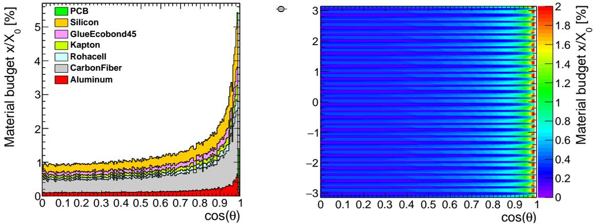
**Figure 3:** Material budget of the inner barrel (left) and its allocation for the full IDEA vertex detector (right).
