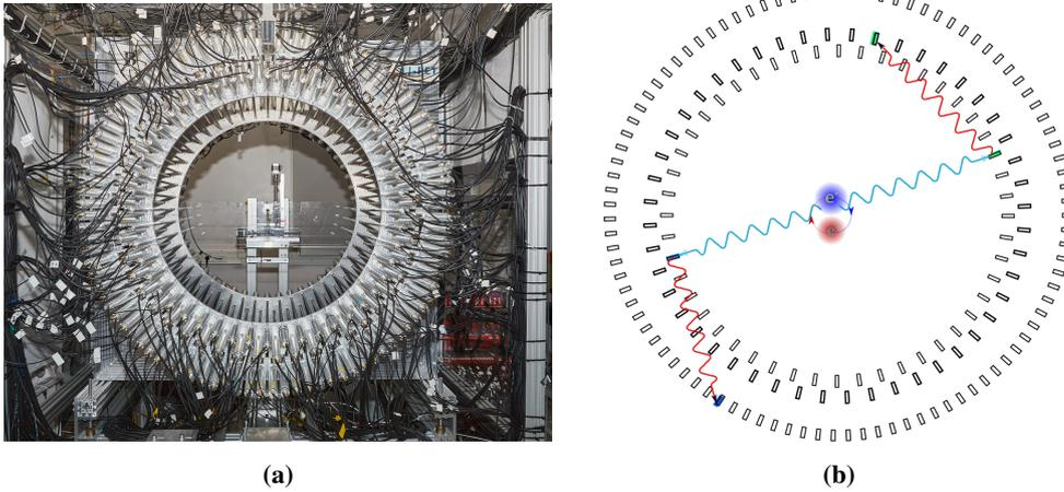
**Figure 1:** (a) The 3-layer J-PET detector in the laboratory. (b) Cross section of the J-PET detector overlapping with event of interest. Electron and positron annihilate in the centre of the detector emitting annihilation photons(Blue lines) and their subsequent scattered photons(Red lines)
