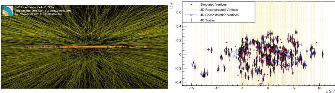
**Figure 1:** Left: Event display of 100-interaction pileup in a 2016 run. Right: Simulated and reconstructed vertices with 200 pileup interactions using a 30 ps timing detector, showcasing 3D-reconstructed vertices, and 4D tracking and vertices. [4]
