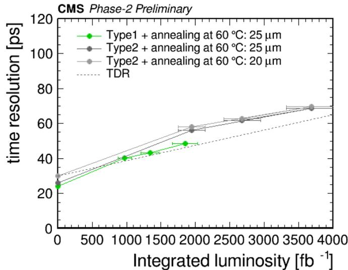
**Figure 6:** Time resolution as a function of the equivalent integrated luminosity (operation at  $T = -45^{\circ}\text{C}$  and SiPM annealing at  $T = 60^{\circ}\text{C}$ ). Data are from test beam measurements of modules (both type 1, in green, and type 2, in grey) with non-irradiated and irradiated SiPMs and tested at various operating temperatures to emulate different points of detector lifetime.
