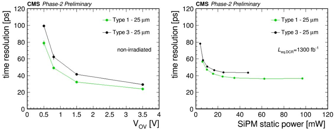
**Figure 5:** Comparison of the time resolution achieved with type 1 and type 3 modules. A better time resolution with thicker modules is achieved both with non-irradiated (left) and irradiated SiPMs (right).
