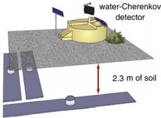
Figure 2: Final design and set-up of the UMD: Three 10\text{ m}^2 modules buried at a depth of 2.3 m and paired to a WCD station located either in the 750 m or the 433 m array.
