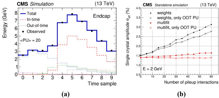
**Figure 2a:** Example of fitted pulses using the multifit reconstruction algorithm, for simulated events with 20 average pileup interactions and 25 ns bunch spacing. **Figure 2b:** Effective resolution for the single crystal amplitude as a function of pileup for the weights and multifit methods.
