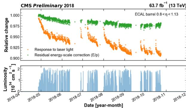
**Figure 4:** Ecal response to the laser lights and the residual energy-scale correction in 2018.
