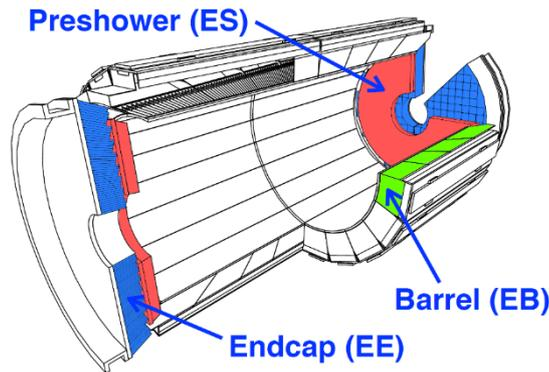
Figure 1: Schematic ECAL layout.
