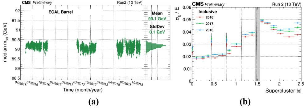
**Fig. 6a:** Time stability of the di-electron invariant mass distribution in Run 2 using  $Z \rightarrow ee$  events. **Fig. 6b:** Relative electron energy resolution as a function of  $\eta$  for different years in Run 2.
