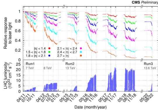
**Figure 3:** Evolution of the ECAL channel response to laser light versus time since 2011. The channels are subdivided in ranges of  $\eta$ . The bottom panel shows delivered instantaneous luminosities.
