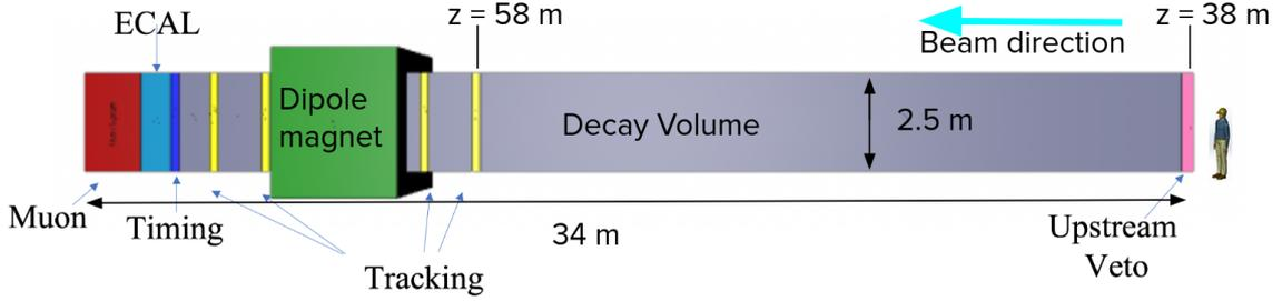
**Figure 3:** SHADOWS detector layout (lateral view). The grey area is the vacuum vessel. The green block is the dipole magnet placed between four tracking stations (yellow)
