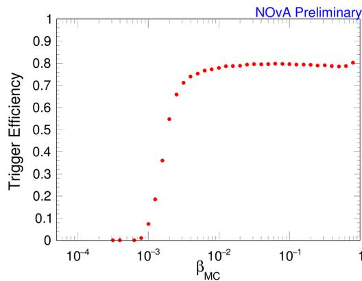
**Figure 2:** This plot shows the trigger efficiency of the fast magnetic monopole trigger.
