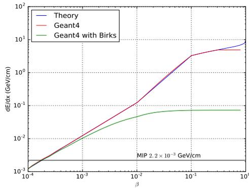
**Figure 1:** This plot shows a comparison of the Geant4 simulated energy deposition model (red) with the theoretical calculations (blue) [2, 3]. The Birks-suppressed energy deposition model in Geant4 is also shown (green). The minimum-ionizing particle (MIP) energy deposition is shown in black for reference.
