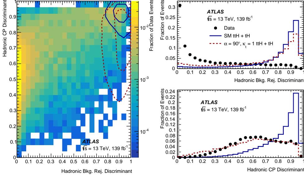
**Figure 4:** Left: two-dimensional BDT distribution in the selected data events ( $m(\gamma\gamma)$  in [105, 160] GeV) from the  $ttH, H \rightarrow \gamma\gamma$  hadronic region showing the Background Rejection BDT and CP BDT. The inner (outer) contours capture 25% (50%) of the  $ttH$  and  $tH$  signal events for CP-even (blue) and CP-odd (red) hypotheses. Right: projections onto the background rejection and CP BDT axes [8].
