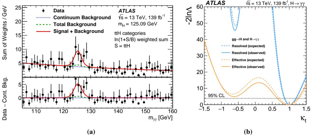
**Figure 3:** (a) Combined diphoton invariant mass distributions for categories targeting the  $ttH$  production processes. (b) Negative log-likelihood scans as a function of  $kappa_t$  in a model where other coupling modifiers are fixed to their SM values. The  $H \rightarrow \gamma\gamma$  and  $gg \rightarrow H$  loops are either parameterized as a function of  $\kappa_t$  (blue) or fixed to their SM expectation (orange) [6].
