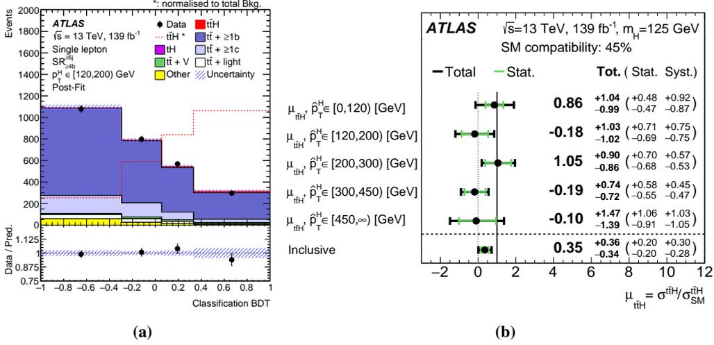
**Figure 1:** (a) Comparison between data and prediction for the BDT discriminant used the single-lepton  $ttH, H \rightarrow bb$  signal region with  $p_T^H < 120$  GeV after the inclusive fit to the data. (b) Signal-strength measurements in the individual STXS  $p_T^H$  bins, as well as the inclusive signal strength [1].
