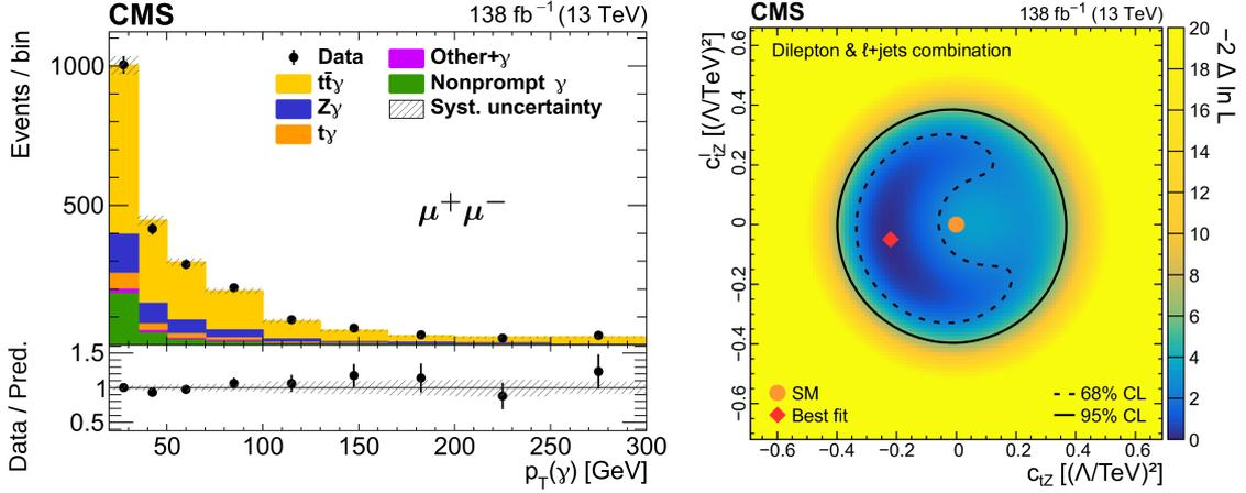
**Figure 1:** Post fit event yields as a function of the reconstructed photon  $p_T$  for the  $\mu^+\mu^-$  channel (left) [6]. Results from the two dimensional scan of the WCs  $c_{IZ}$  and  $c_{IZ}^I$  using the combination of the reconstructed photon  $p_T$  in the dilepton [6] and the  $\ell$ +jets [9] channels (right).
