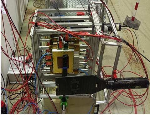
**Figure 5:** MM and Scintillator based setup for muon background measurement
