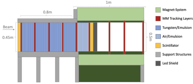
**Figure 1:** Side schematic of the NaNu with its four major components [1]
