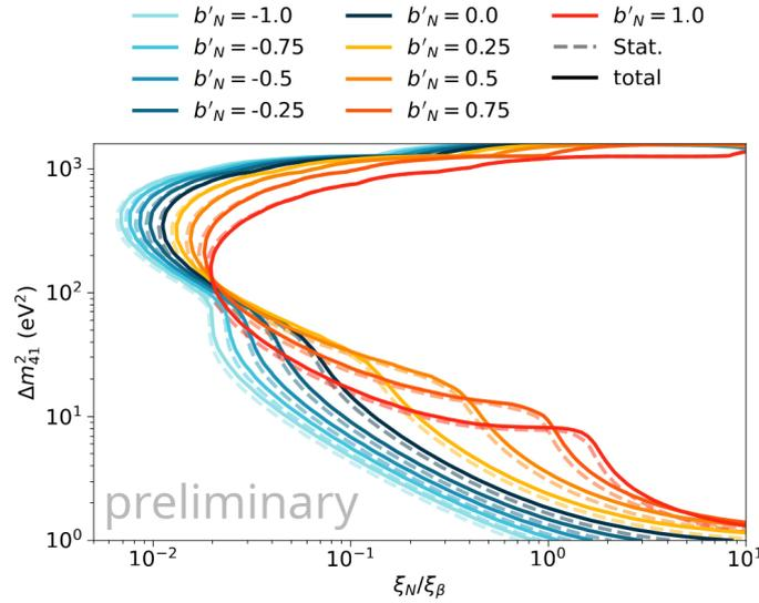
**Figure 2: GNI sensitivity contour considering an additional right-handed neutrino at 95 % CL, taking into account systematic effects. The study was performed on simulated data of the KATRIN campaign.**
