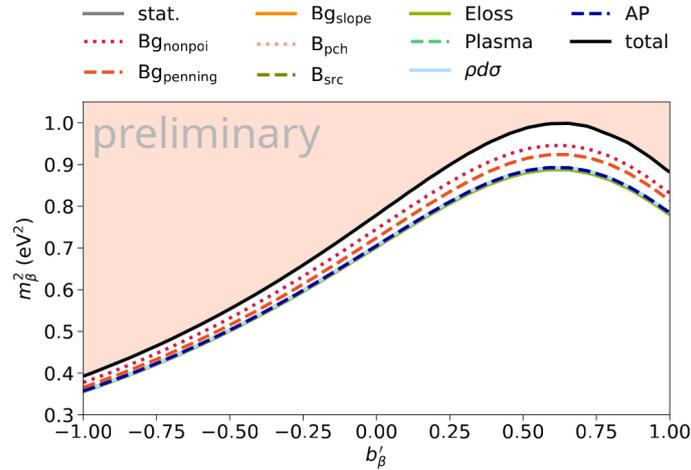
**Figure 1: GNI sensitivity contour considering only a left-handed neutrino at 95% CL, taking into account different systematic effects. The study was performed on simulated data of the KNM2 campaign.**
