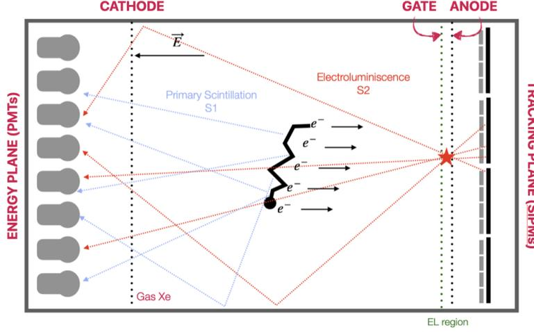
Figure 1: Graphical representation of the NEXT asymmetric HPGXe-EL TPC.
