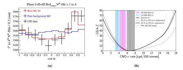
**Figure 1:** (a) CID best fit illustration (red) and a pure background hypothesis (blue) for the first 4 hits in all phases. (b) Likelihood profile of the CNO- $\nu$  rate from spectral fit using the CID constraint without (black dotted) and with (black solid) systematic errors. Grey dashed line shows the profile without the CID constraint [5, 9].
