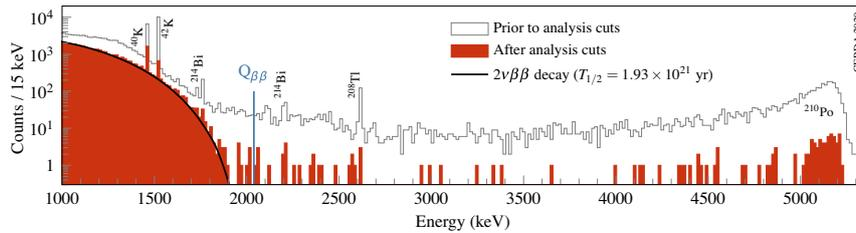
**Figure 1:** GERDA Phase II energy spectrum in the 1 to 5.3 MeV region before and after the analysis cuts. The  $Q_{\beta\beta}$  and the prominent  $\gamma$  lines and  $\alpha$  decays around 5.2 MeV are shown. Taken from [5].
