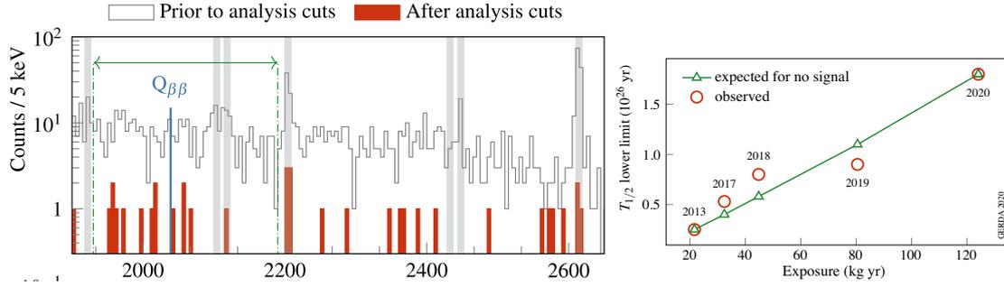
**Figure 2:** Left: GERDA Phase II enlarged energy spectrum in the 1900 - 2650 keV region, before and after the analysis cuts. The regions of expected  $\gamma$  lines are marked in grey. Right: lower limit (90% C.L.) on the  $0\nu\beta\beta$  decay half-life of  $^{76}\text{Ge}$  as a function of the exposure. Taken from [5].
