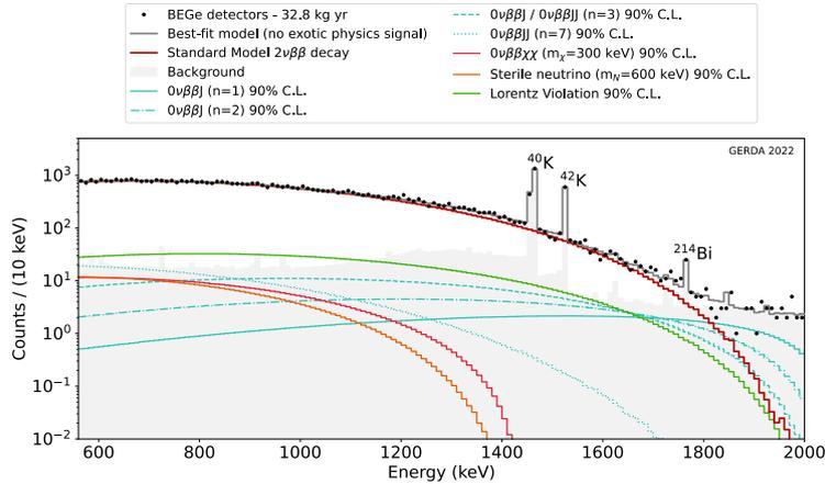
**Figure 4:** Data energy spectrum and best-fit model, corresponding to the absence of any new physics signal. Taken from [8].
