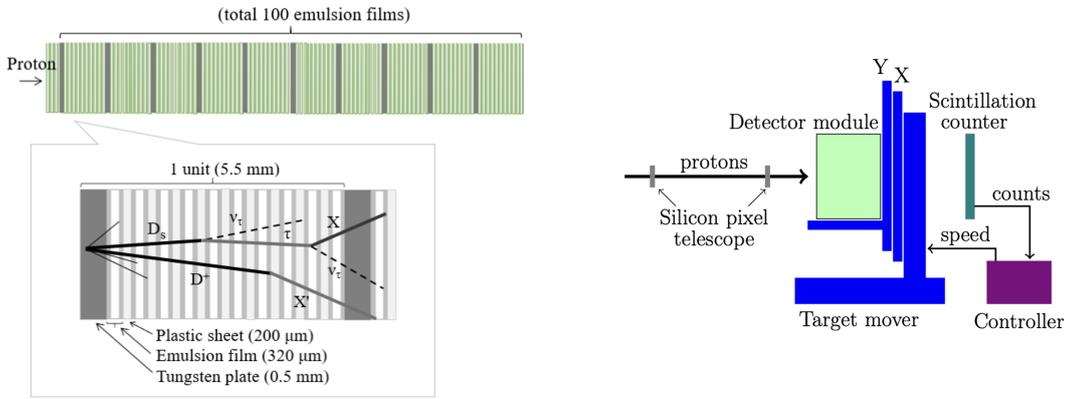
**Figure 2:** Left: schematics of the DsTau detector. Right: a drawing of the target mover.
