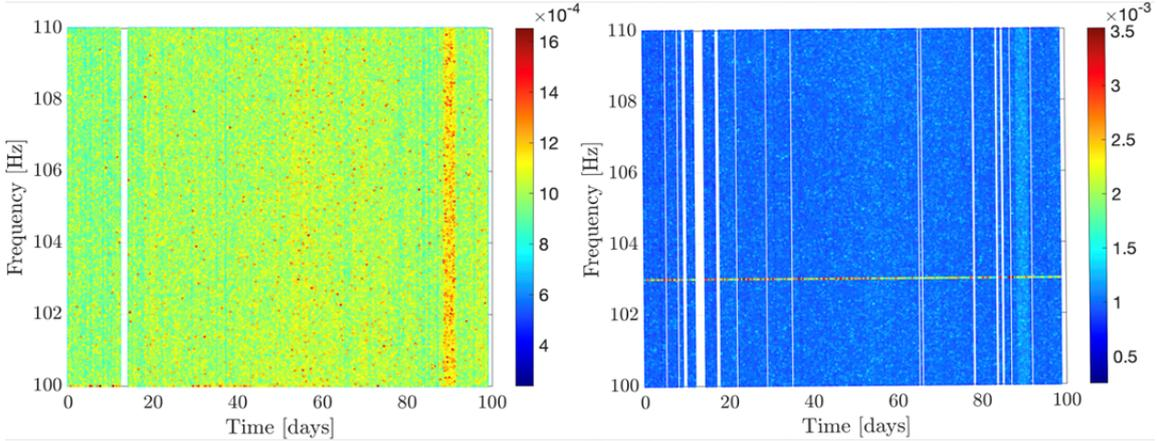
**Figure 1:** Peakmap of an injected signal with a chirp mass of  $10^{-4} M_{\odot}$  at 1 kpc and with a reference frequency of 103 Hz with no correction (left) and after the heterodyne correction (right) with O3b data of LIGO Livingstone. The colorbar shows the amplitude of the FFT transform in 1/Hz. The time is expressed with respect to the initial time of O3b, 1st of November of 2019 at 15:00 UTC.
