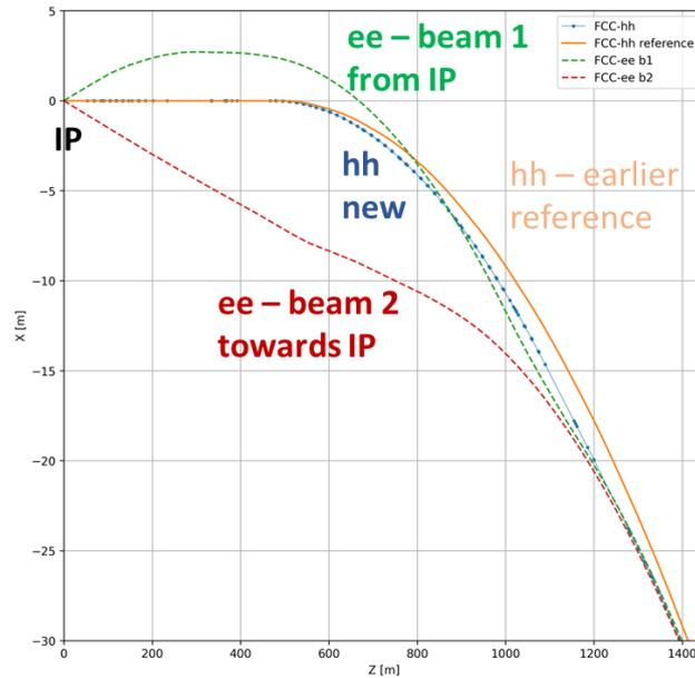
**Figure 9:** Three-beam footprint around an interaction point, before and after final FCC-hh interaction-region optics adjustment (Courtesy T. Risselada, M. Giovannozzi, and G. Pérez Segurana).
