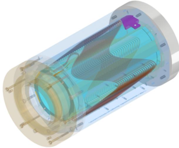
**Figure 3:** CAD design of HTS sextupole demonstrator based on canted  $\cos\theta$  coils (Courtesy M. Koratzinos).
