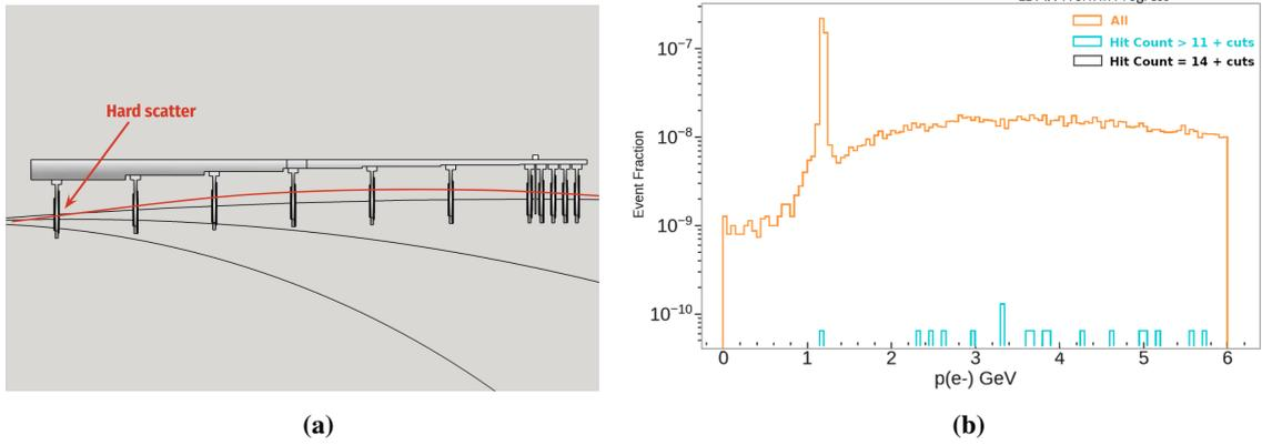
**Figure 3:** (a) Sketch of an example of an off-beam-energy electron traversing the tagger tracker. (b) Reconstructed momentum for off-beam electrons for various track quality selections.
