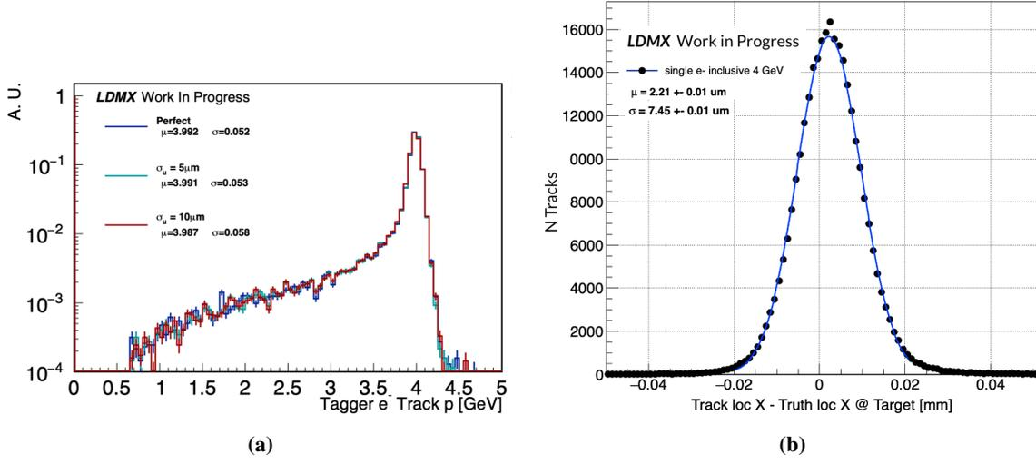
**Figure 2:** (a) Momentum distribution for beam  $e^-$  reconstructed in the tagger tracker for  $E_{beam} = 4$  GeV for perfect measurements and with  $5\mu\text{m}$  and  $10\mu\text{m}$  hit-smearing factors. (b) The residual between the local-x position of the tracks with the Geant4 particles at the target surface.
