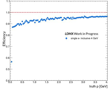
**Figure 4:** Reconstruction efficiency for a *findable* recoil electron particle.
