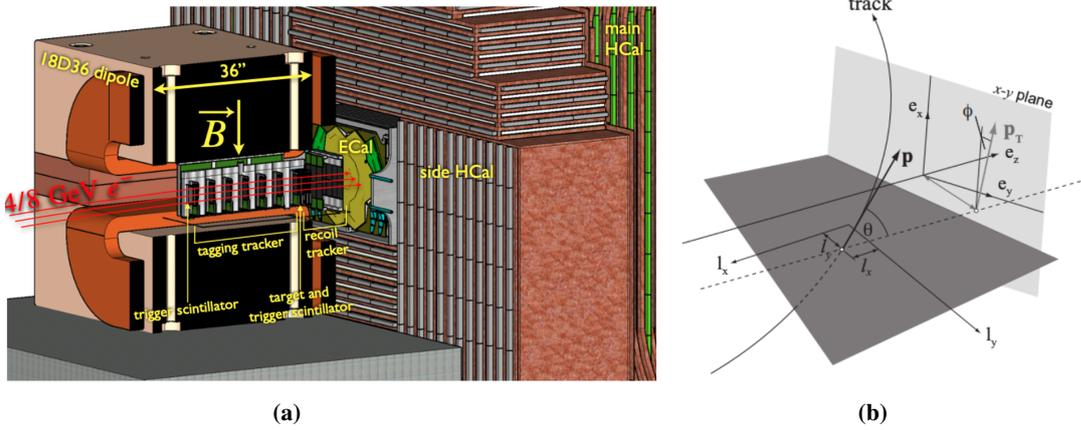
**Figure 1:** (a) The LDMX detector concept. (b) Track parameters on a detector or target surface.
