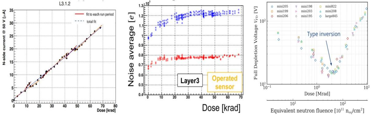
**Figure 4:** Left plot: Leakage current as a function of the accumulated dose; Center plot: the average noise level as a function of the accumulated dose for the *p*-side (blue dots) and *n*-side (red dots); Right plot: full depletion voltage as a function of the accumulated dose with the type inversion observed at 2 Mrad.
