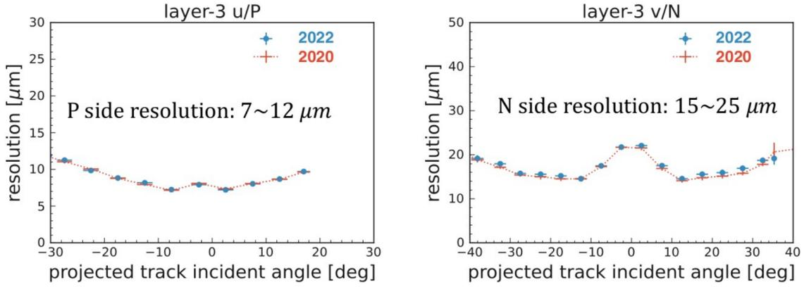
**Figure 3:** Distributions of position resolution for *p*-side (left) and *n*-side (right) as a function of the track incident angle. A comparison between data taken in 2020 (dots) and 2022 (dotted lines) is presented.
