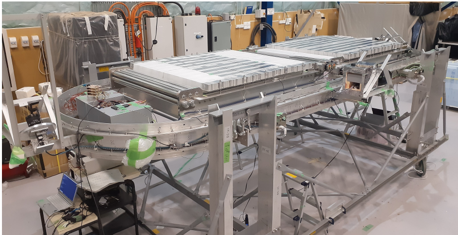
Figure 7: Emulsion telescope after installation of the converter films. Two roller-driven multistage shifters are mounted on the pressure vessel gondola, and all 20 converter packs are mounted there. The total sensitive area is 2.5 \text{ m}^2 ( 1.25 \text{ m}^2 \times 2 sets). The controller, communication equipment, and batteries for each device are mounted in both semicircles.
