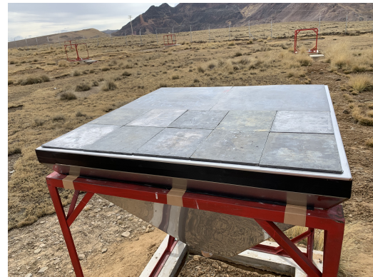
(b) The photo shows a scintillator counter with 0.5 cm thick lead plates on the top of the detector. The detector is supported by an iron structure, which is secured to a concrete base. Additionally, there is a stainless steel pyramidal structure that is 1 mm thick, which is also held by the iron structure.
