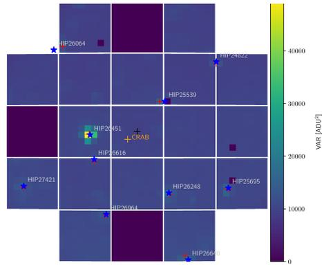
**Figure 4:** Variance image relative to a Crab observation with ASTRI-Horn; red crosses represent the reconstructed position of the stars indicated by blue stars. The angular size of a PDM is  $1.5^\circ \times 1.5^\circ$
