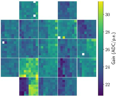
**Figure 3:** Map of the ASTRI-Horn SiPMs gains derived from pulse-height distribution spectra obtained using the internal camera calibration system.
