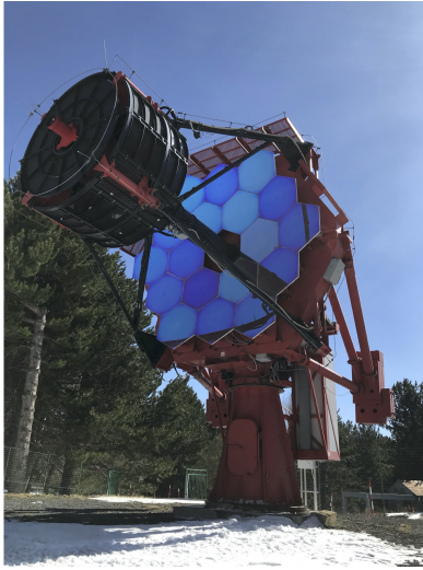
Figure 3: ASTRI-Horn at the INAF SLN station after the installation of the new 18 segments of M1.
