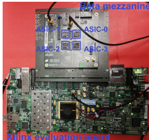
Figure 9: Picture of the Xilinx EK-Z7-ZC706-G evaluation board configuring and controlling a Beta mezzanine hosting four Beta ASICs.
