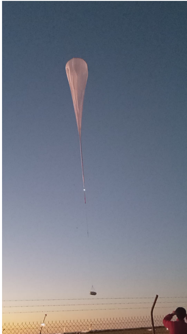
Figure 4: The balloon at the time of launch (about 6:30 a.m. local time). The balloon is approximately 130 meters from the head to the tail (mid-light point) (volume of 300,000 cubic meters when fully inflated in the sky). The gondola weighs about 1.1 tons (ballast about 0.4 tons), and the total weight including the balloon is about 1.9 tons.
