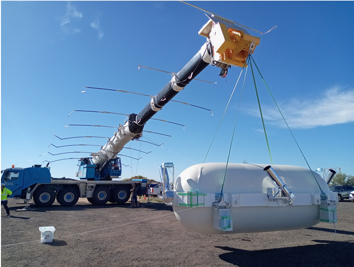
Figure 3: After closing the pressure vessel shell, during final engagement, the silver cylinder facing in three directions is the stray light hood of the star camera.
