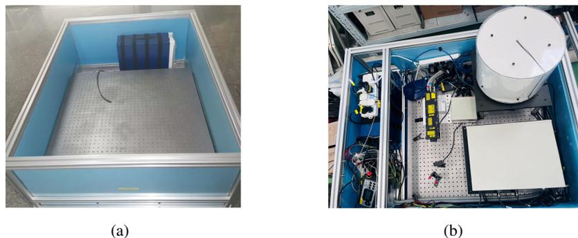
**Figure 3:** (a): The aluminum alloy framework of the laser calibration system, indicated by the blue portion, is insulated with insulating material, the insulation layer used to divide the cavities in the figure is temporarily removed. Acrylic panels are fixed on the outer side of the frame as a protective layer; (b): The schematic of the laser calibration system.
