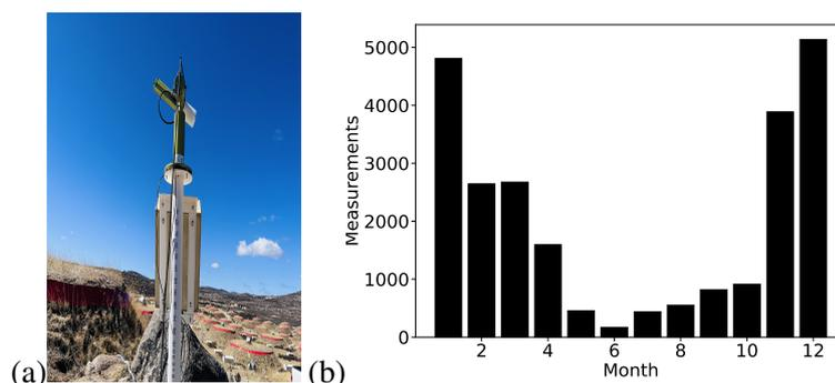
**Figure 2:** (a) CE-318T in the field observations. (b) The number of measurements VS month, some months may have less data because of the cloudy weather
