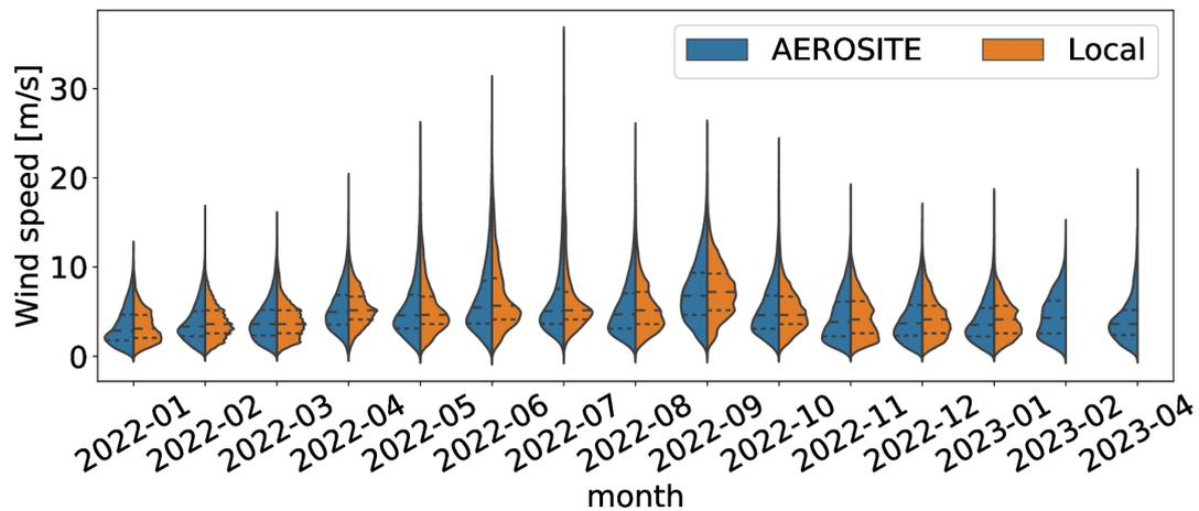
**Figure 5:** Monthly distributions of wind speed in the AEROSITE data and data from a local weather station.
