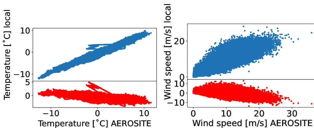
**Figure 6:** Correlation of the nearest measurements of temperatures (left) and wind speeds (right) in the AEROSITE data and data from a local weather station. The lower red subplot shows differences of individual values.
