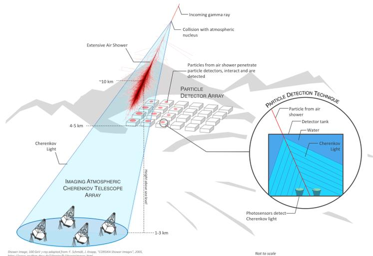
**Figure 1:** Gamma-ray detection illustration (courtesy of SWGO).
