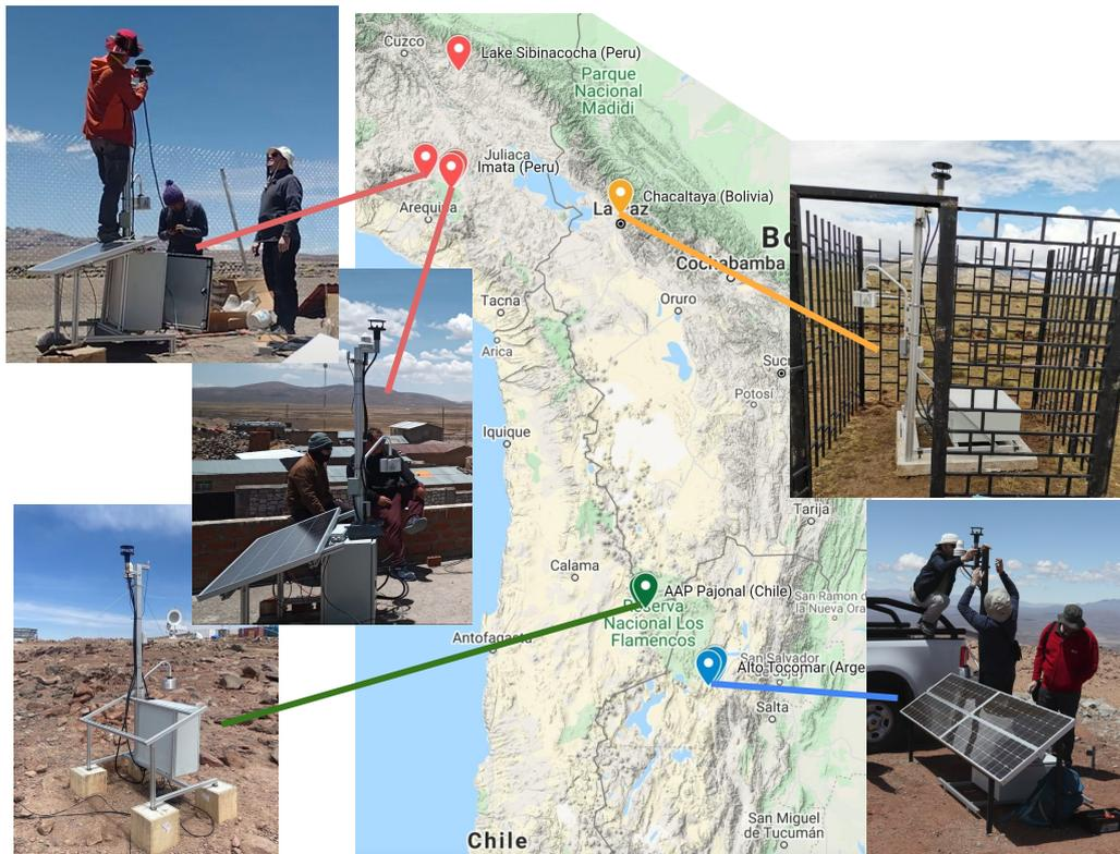
**Figure 3:** Locations and site photos of deployed AEROSITES. The Peruvian AEROSITE deployed at Imata was moved to Yanque in Oct 2022.
