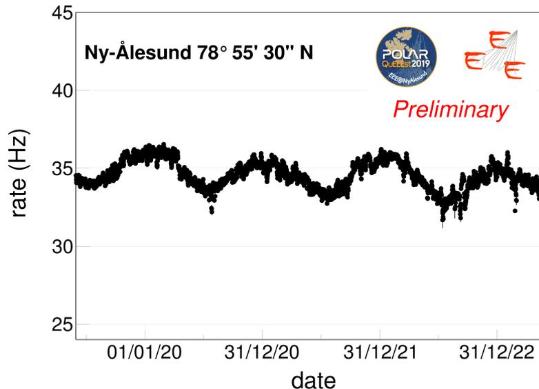
**Figure 3:** Muon flux as measured by the PolarquEEEst detectors at Ny-Ålesund in the period 2019-2023.
