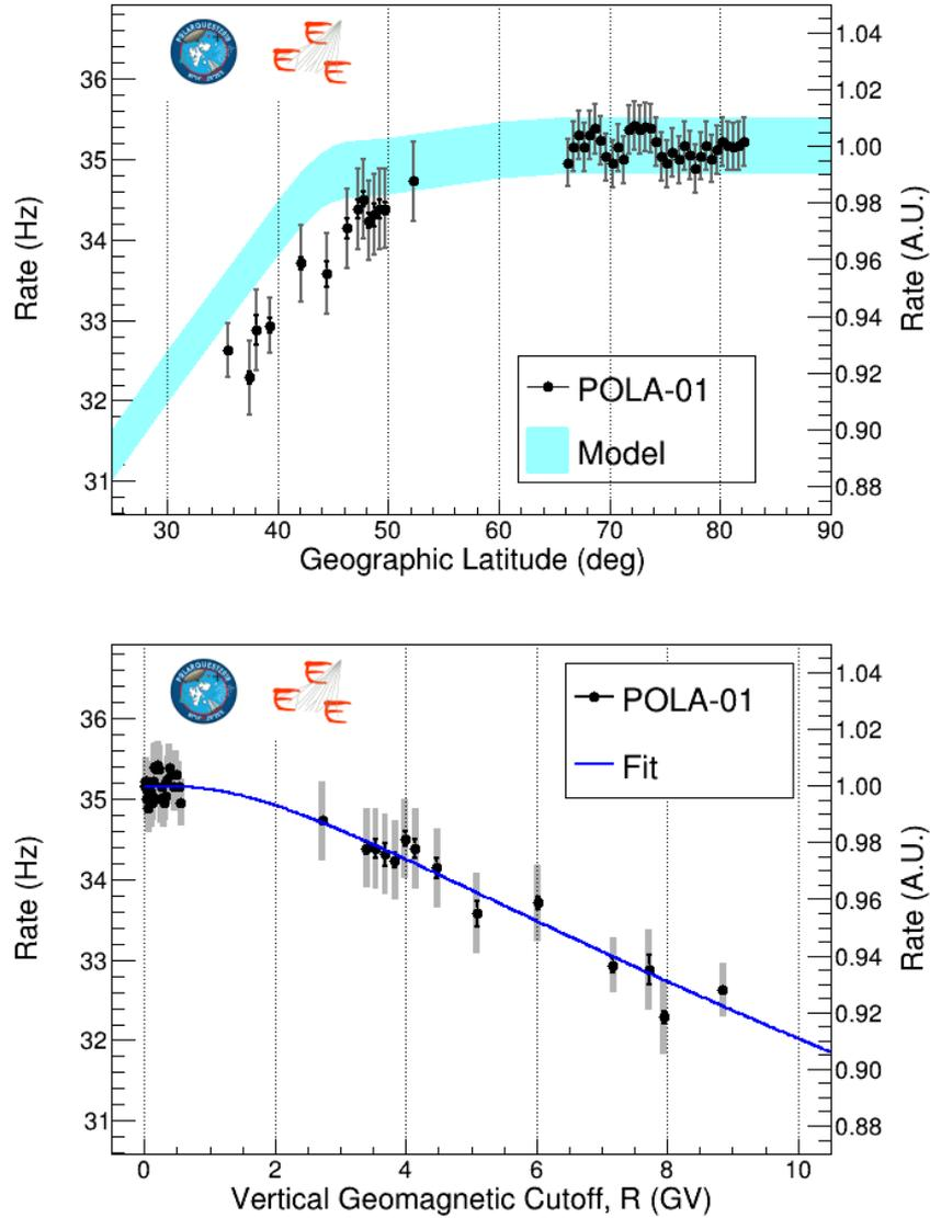
**Figure 2:** Cosmic particle rate measured by the POLA-01 detector as a function of the geographic latitude (top panel), and as a function of the vertical geomagnetic cutoff (bottom panel) [6].
