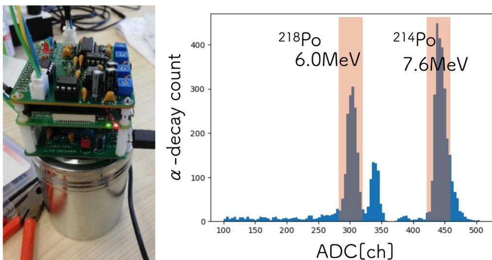
**Figure 3:** (Left) Radon detector developed by students. (Right) Measurement of  $\alpha$ -decay from daughter nucleus of radon in the rock.
