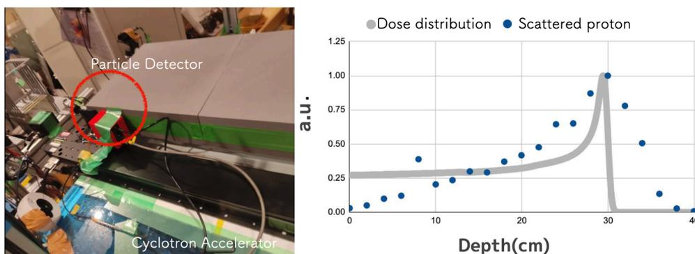
**Figure 4:** (Left) Proton irradiation using the AVF cyclotron accelerator at CYRIC, Tohoku University. The detector was moved along the phantom to obtain the dose distribution due to scattered protons. (Right) Measured values are shown as blue dots, and the solid gray line shows the dose distribution calculated by a Monte Carlo simulation code called PHITS.
